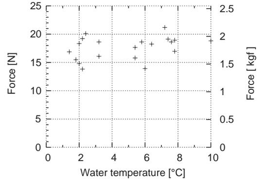
Fig. 2. Temperature - bonding strength comparison. X-axis: water temperature  $[\text{ }^\circ\text{C}]$ , Y-axis: force to detach  $[\text{N}, \text{kgf}]$
