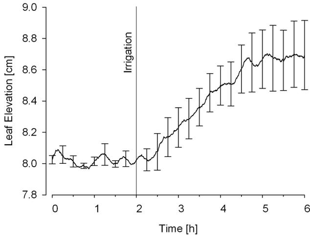
**Fig. 2:** The average normalised vertical movement of the canopy after an irrigation event with 50 ml of water, measured with the sensor disc (n=8).
