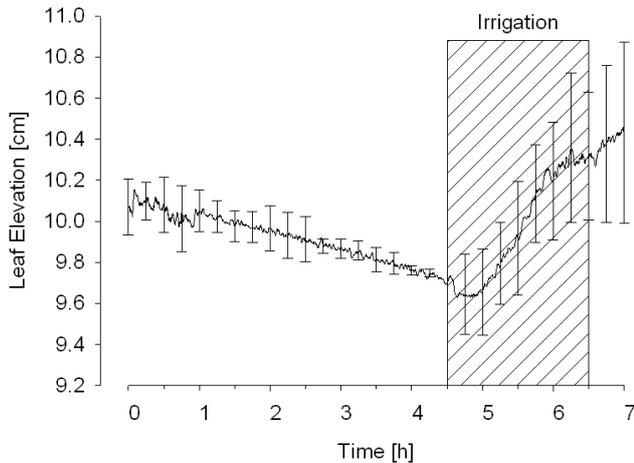
**Fig. 4:** The average normalized leaf inclination signal in autonomous irrigation ( $n=5$ ).
