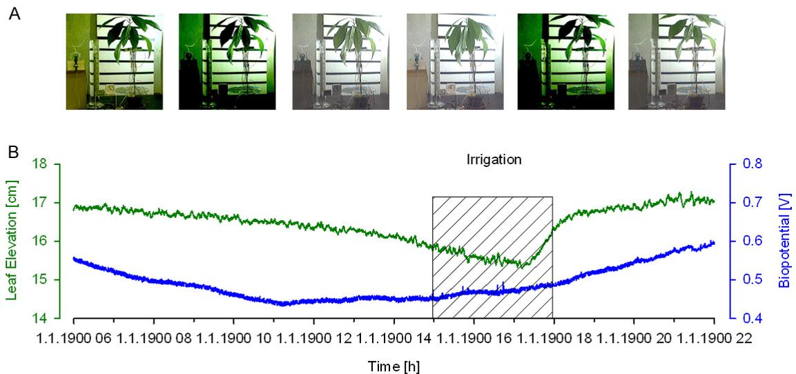
**Fig. 5:** (A) Time series of pictures showing morphological changes of an avocado plant during an automatic irrigation experiment with increased detection threshold. (B) Plot of the average leaf elevation and the biopotential during the close-loop experiment.
