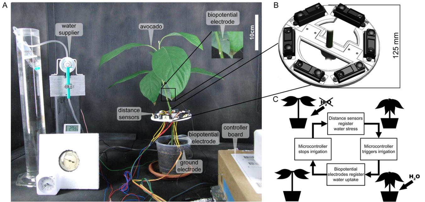
**Fig. 1:** (A) Snapshot of the whole experimental setup. (B) The disc that supports the six distance sensors which compose the leaf inclination detection system. (C) Schematic of the closed-loop interaction to which the experiments should lead.
