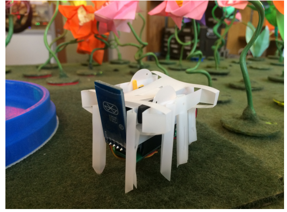
Fig. 3. An insect manufactured using print-and-fold techniques can crawl around the flowers.
