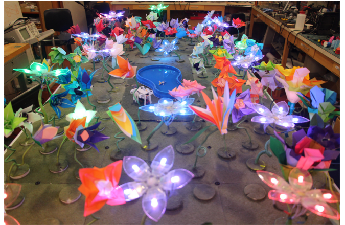
Fig. 1. The Robot Garden is a heterogeneous collection of distributed robots, including 100 actuated origami flowers and mobile foldable insects.
